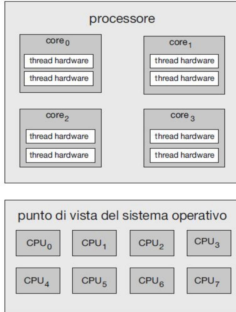
Figura 5.14 Chip multithreading.
